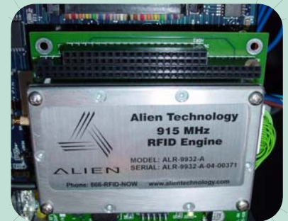
RFID Module is Easy to Add At anytime through standard PC104 expansion port inside LA/4500 unit
