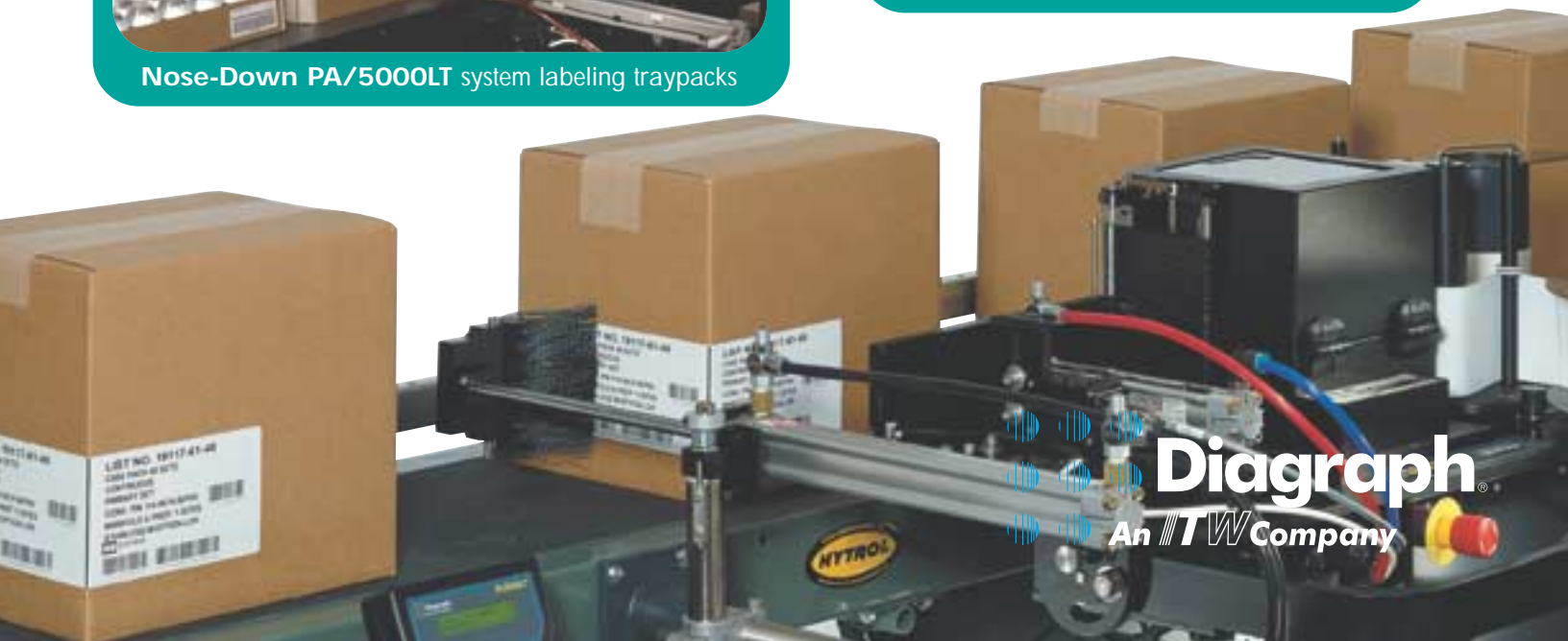
PA/5000LT equipped with front apply swing arm
