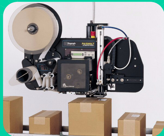
FAST! System Can Print, Program, Apply and Verify 50 PPM with a 4x6 Label
