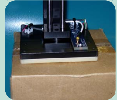
TampTenna™ Programs and Verifies RFID Labels
