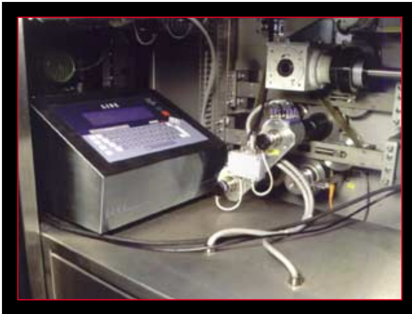
Each of the two ink jet coders has its own control panel embedded right in the hot-pack cheese wrapping machine.
