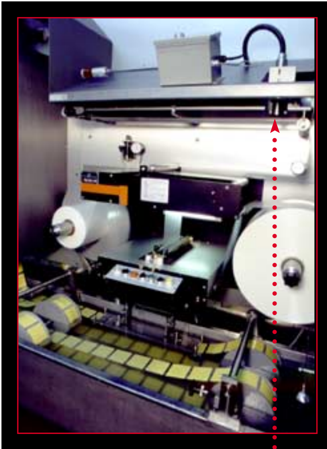
Film is ink jet coded prior to filling at speeds of 250 fpm.
