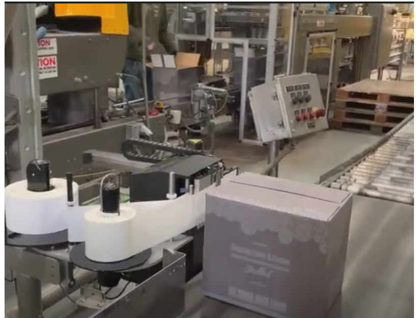
The Diagraph all-electric PA7100 applies labels to cases at Don Sebastiani & Sons
