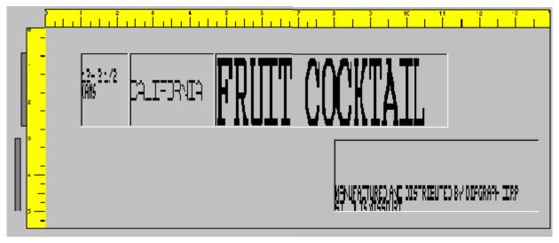
The screen below shows the three messages from the upper printhead with Message Frames around each message. The spacing between the end of message one and the beginning of message two is created by spacing at the end of the first printed line in message 1 (12-2  $\frac{1}{2}$ ).
