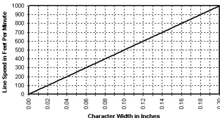
Minimum Character Width for a Given Line Speed
