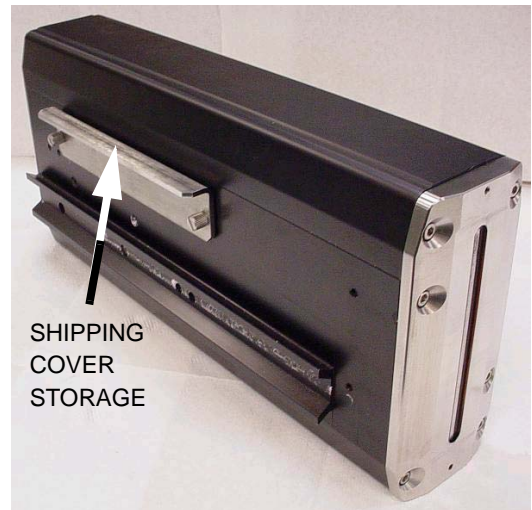
LOOSEN TWO CAPTIVE THUMB SCREWS TO REMOVE SHIPPING COVER
