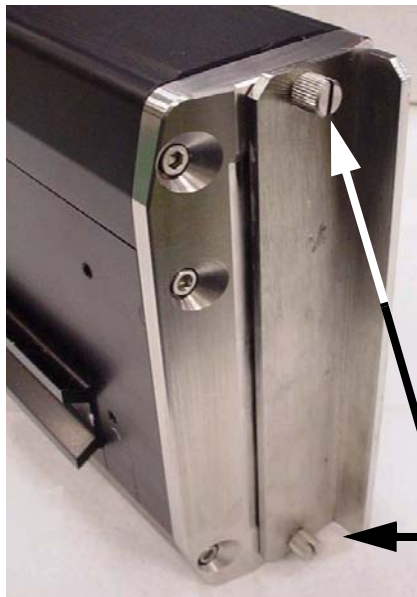
LOOSEN TWO CAPTIVE THUMB SCREWS TO REMOVE SHIPPING COVER
