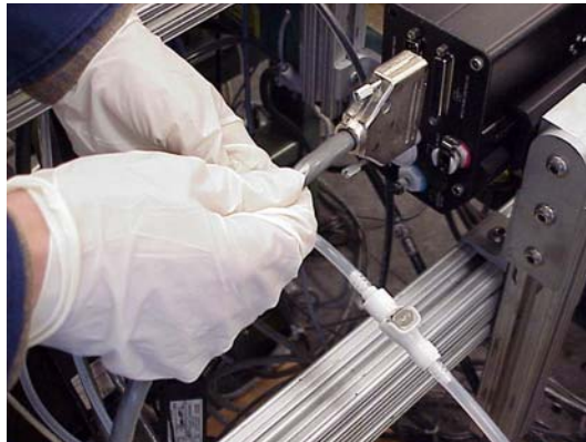
BEFORE PRINT HEAD CABLE IS CONNECTED AND INK TUBING IS BLED
